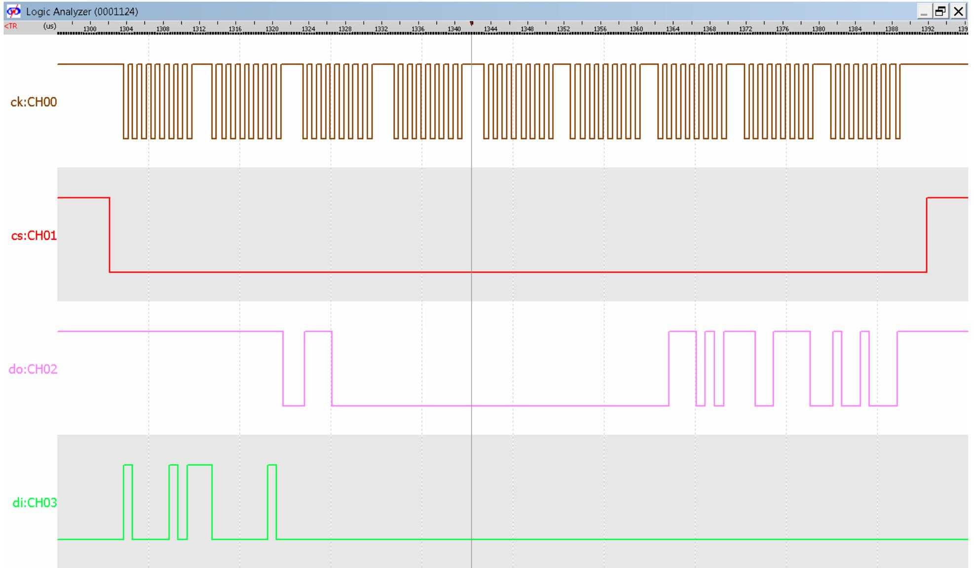
Read data captured in 6802 through sub-20 (logic analyzer inputs at 6802 pins)
