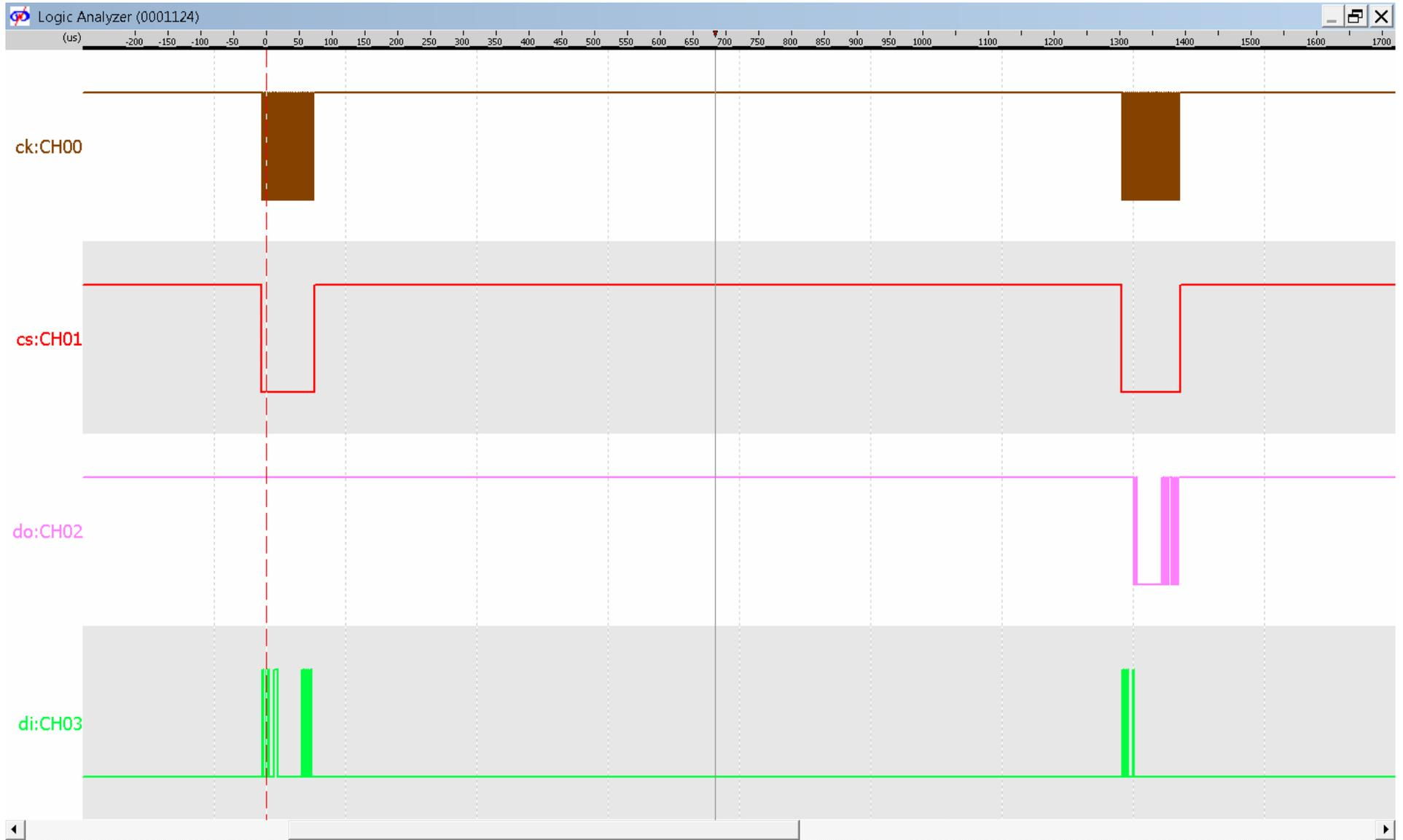
Complete write and read to 6802 transaction through sub-20
